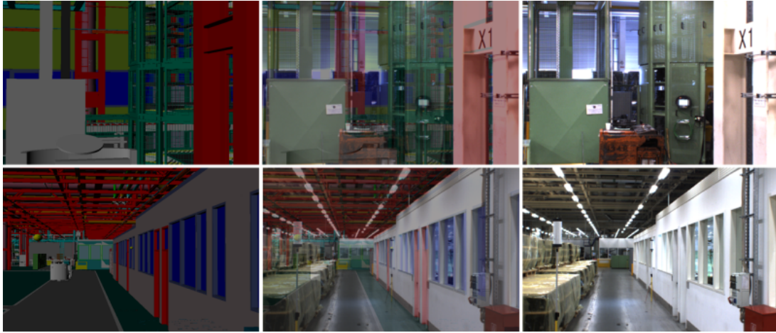
Figure 4: Evaluation of the system in a factory. The virtual, overlayed and video image are shown.
